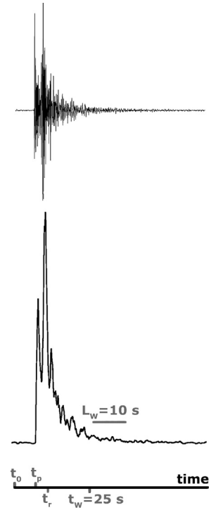
Fig. 3. Seismic time measurements. An example velocity waveform and envelope with corresponding time-related quantities as defined in the study.
